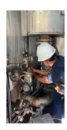
Collecting real-time surface temperature readings to validate the value of granular temperature data in understanding steam consumption for a dyeing machine in a textile manufacturing plant in Malaysia.
