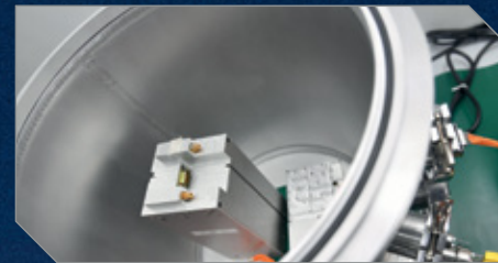
A vacuum chamber is used to simulate the space environment to stress-test the electronics design of the IDRS terminal.
