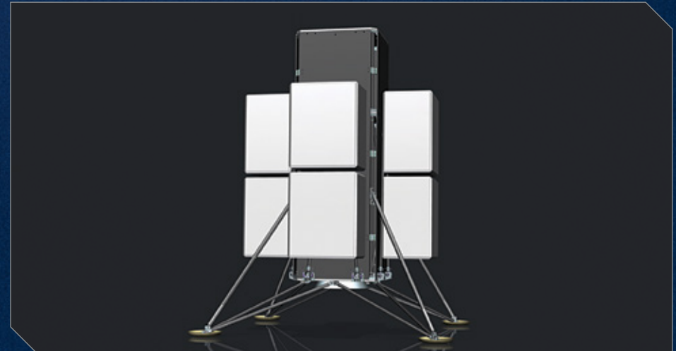
Equipped Primary Structure Central Tube of the Qosmosys Moon Lander (QML).
