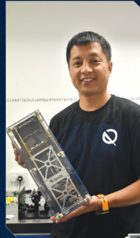
SpeQtral co-founder and CEO Chune Yang Lum holding the CubeSat SpooQy-1, which was the first to demonstrate a miniaturised source of entangled photons in space.
