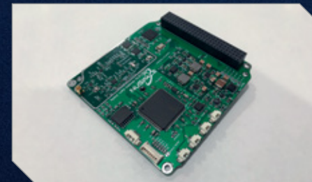
The Space LoRa Gateway, which was developed in-house and enables affordable IoT connectivity in remote areas.
