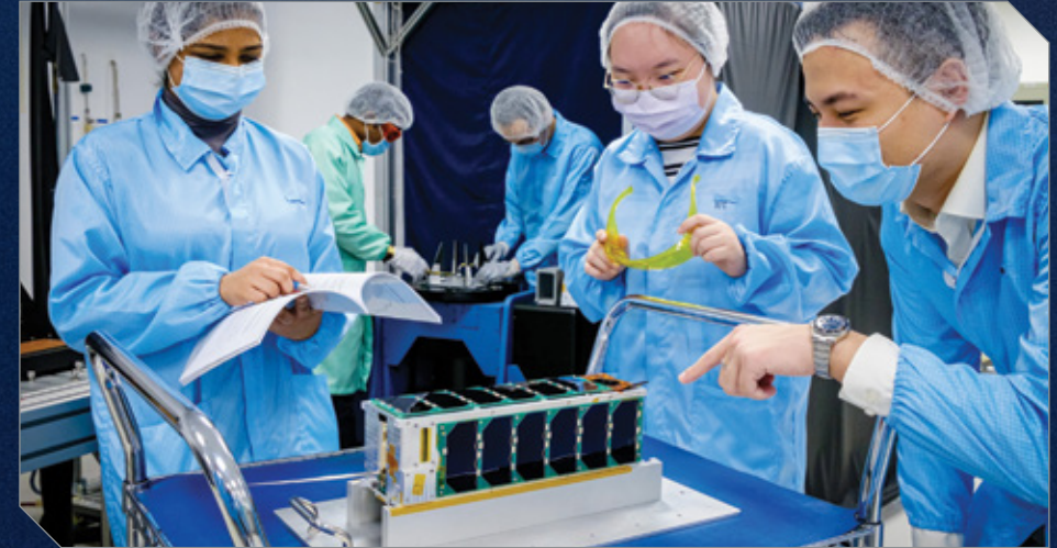
Students preparing the nanosatellite for a final check of its Attitude Determination & Control System in a Helmholtz cage.
