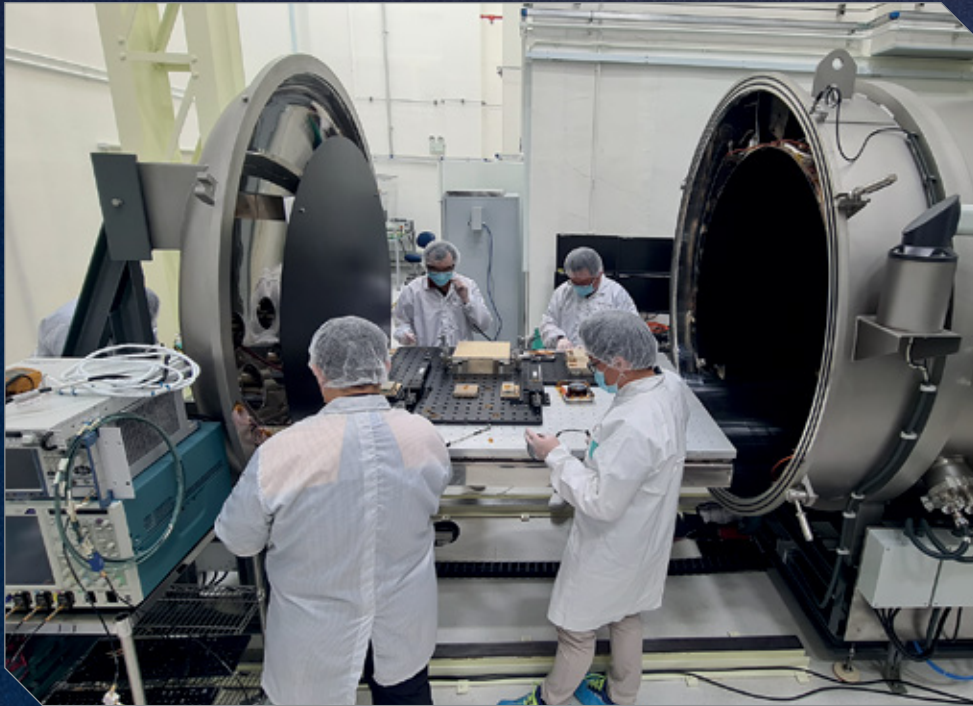
Payload qualification activities for DSO National Laboratories' NeuSAR satellite at ST Engineering Satellite Systems' thermal vacuum facility.
