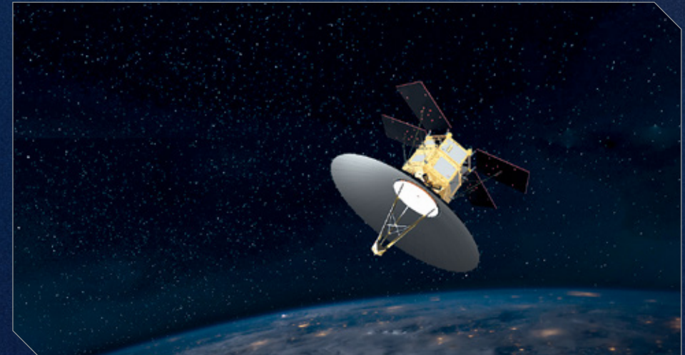
TeLEOS-2, a Synthetic Aperture Radar (SAR) earth observation satellite, is set to launch in 2023.
