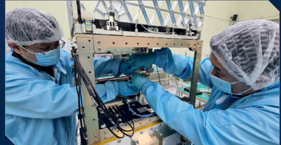
DSO researchers working on the integration of NeuSAR sub-systems.
