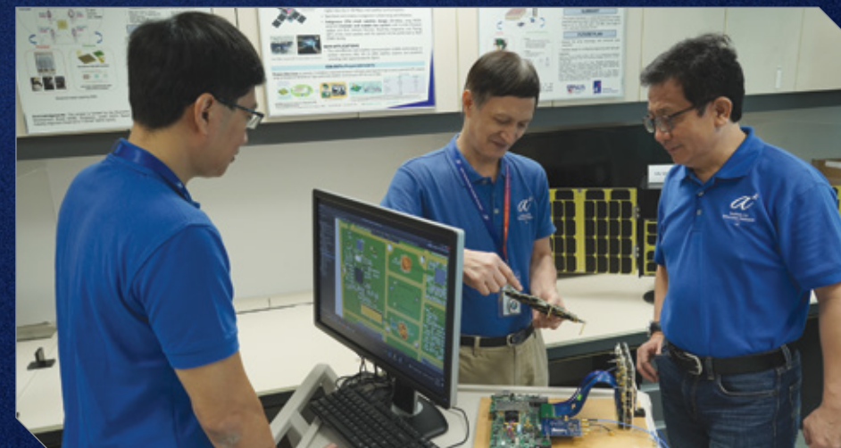
I 2 R researchers performing tests on the Ka-band antenna array for inter-satellite link.
